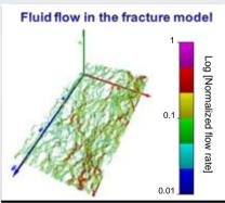
A X-ray CT based numerical analysis of fractured core samples has been developed, providing insights into fracture flow characteristics in reservoirs.
